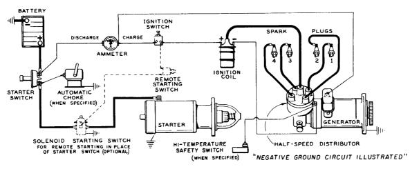
Fig. 12, BATTERY IGNITION - WIRING AND TIMING DIAGRAM
