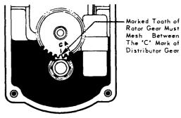
Fig. 2, INTERNAL TIMING GEARS
