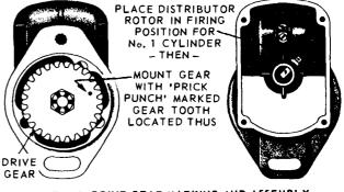
Fig. 3, DRIVE GEAR MARKING AND ASSEMBLY
