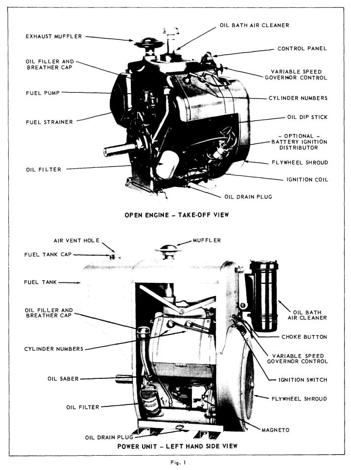
MODEL VG4D OPEN ENGINE AND POWER UNIT
