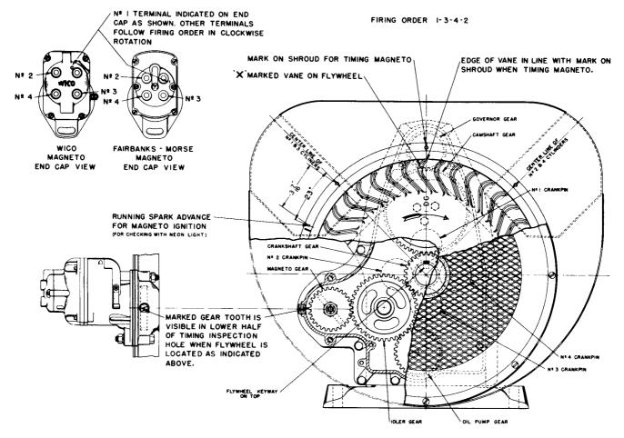
Fig. 11, MAGNETO TIMING DIAGRAM
