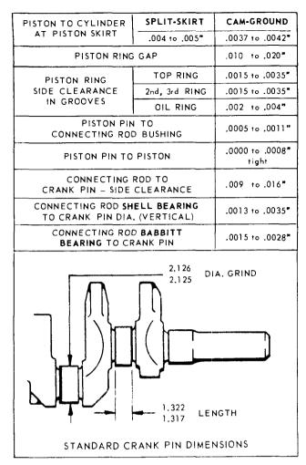
Fig. 34, PISTON, RING AND ROD CLEARANCES CHART
