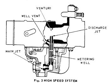
the sizes of the discharge jet orifice, the size of the main jet, and the size of the well vent. The well vent is located in the air intake and permits air to enter the top of the metering well around the outside of the discharge jet. The flow of fuel through the main jet is controlled by the size of main jet opening.
