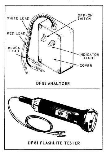
The DF 83 Analyzer was developed for testing the solid state ignition and flywheel alternator components as furnished on *Wisconsin* engines. It is very efficiently and economically powered by four transistor radio type 9 volt batteries. The DF 81 Flashlite Tester is used primarily for checking continuity.
