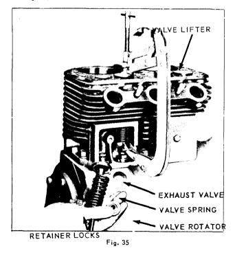
The cylinder blocks do not have to be removed unless the cylinder bore is scored, out-of-round, or worn oversize more than 0.005 inch. In this event, the block will have to be removed, rebored and fitted with over-
