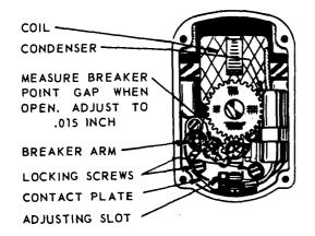
Fig. 1, BREAKER POINT ADJUSTMENT
